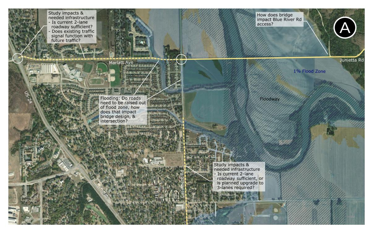
General bridge location based on Floodway width. Exact crossing location is flexible.
