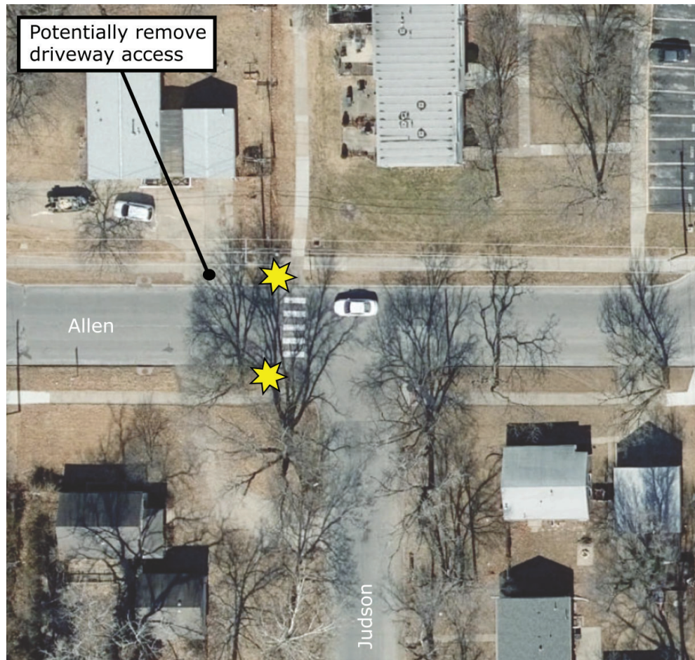
Figure N14. Proposed RRFB installation.
