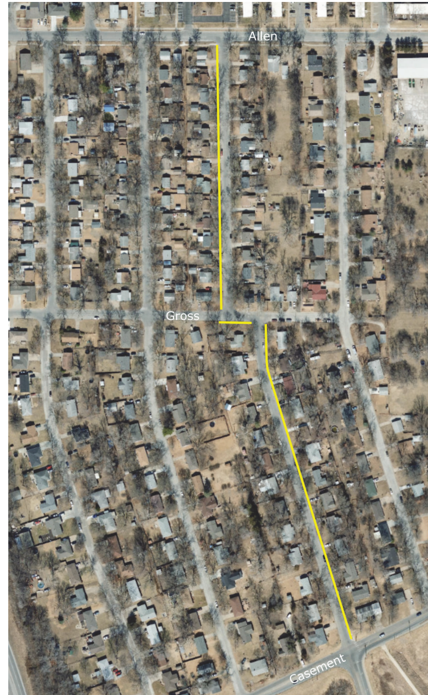
Figure N22. Proposed sidewalk installation.
