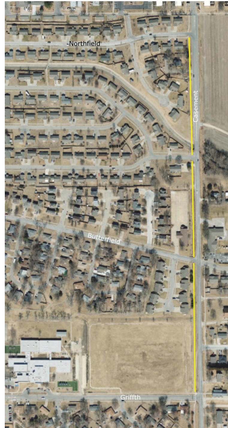
Figure N24. Proposed sidewalk installation.
